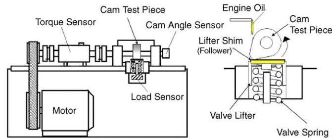
Fig. 5. Single cam and follower test rig.
